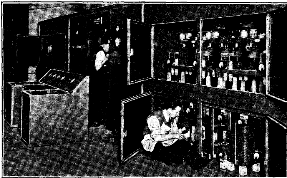
HOLY LAND STATION. The three main panels and control desk of the 20 kW transmitter, nearing completion at the Chelmsford works of the Marconi Co. in readiness for final tests prior to shipment to Palestine for the chosen site, seven miles north of Jerusalem.
