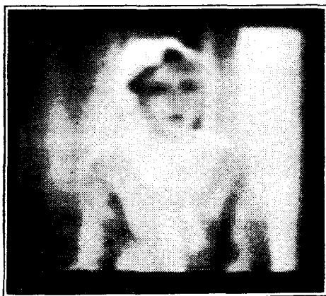
Blurred effect due to the electron lens being out of focus (wrongly adjusted electron lens potential).
