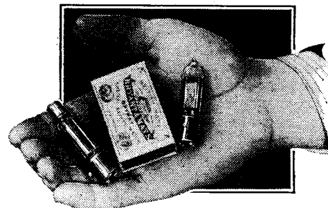
The new miniature valves; the screen grid type is seen on the left.
